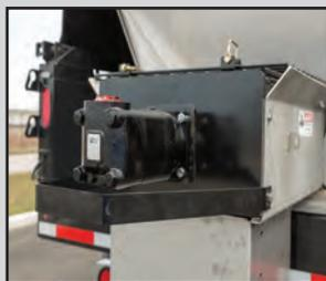
High Torque Auger Motor
