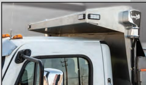
Cab shield with Built-In Tarp System
