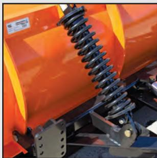
3-1/2" x 3-1/2" x 5/16" Structural steel tubing push frame is 90" wide, running gear mounts are standard
