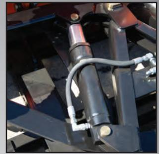
Twin 3" single acting chrome plated hydraulic cylinders for heavy duty power reversing. Located above the push frame for protection & ease of service
