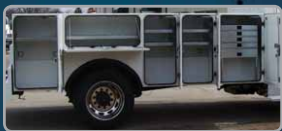
44.5" high compartments with large door clearance provide ample storage space and easy access to tools and equipment (optional Drawer package pictured above)
