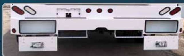
Optional storage bumper features dual locable compartments, factory installed L.E. D. light kit, twin steps and recess for optional hitch package
