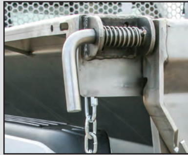
3/4" Diameter stainless steel tailgate hitch pins
