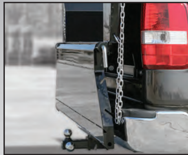
Double pivoting & removable tailgate
