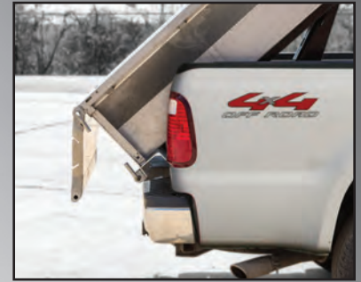
Double pivoting & removable tailgate
