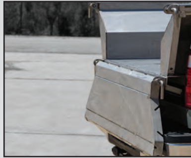
Double pivoting & removable tailgate
