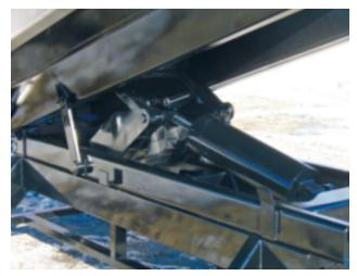
The Underbody Hoist is a solid design Class 50 Series, that combines solid reliability with superior load lifting power. The 1/4" trapezoidal longitudinals support the 1/4" crossmemberless floor.
