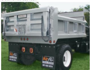
The exceptional durability of the *Pro-Max*° is enhanced by the standard 6-panel tailgate, full depth rear corner posts, and fully enclosed front posts.
