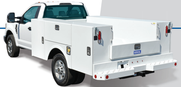
Body pictured with optional Recessed Punched Bumper with surface-mounted LED 3-in-1 Body Light Kit and Aluminum Fuel Fill
